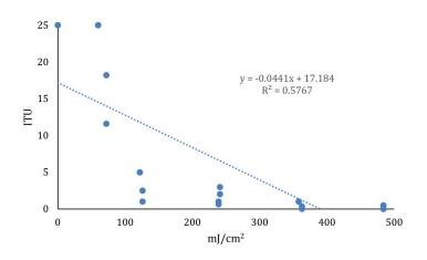
Figure 2: Ichthyotoxic Units (ITU) at Two Hours, Varying HOD UV Doses
